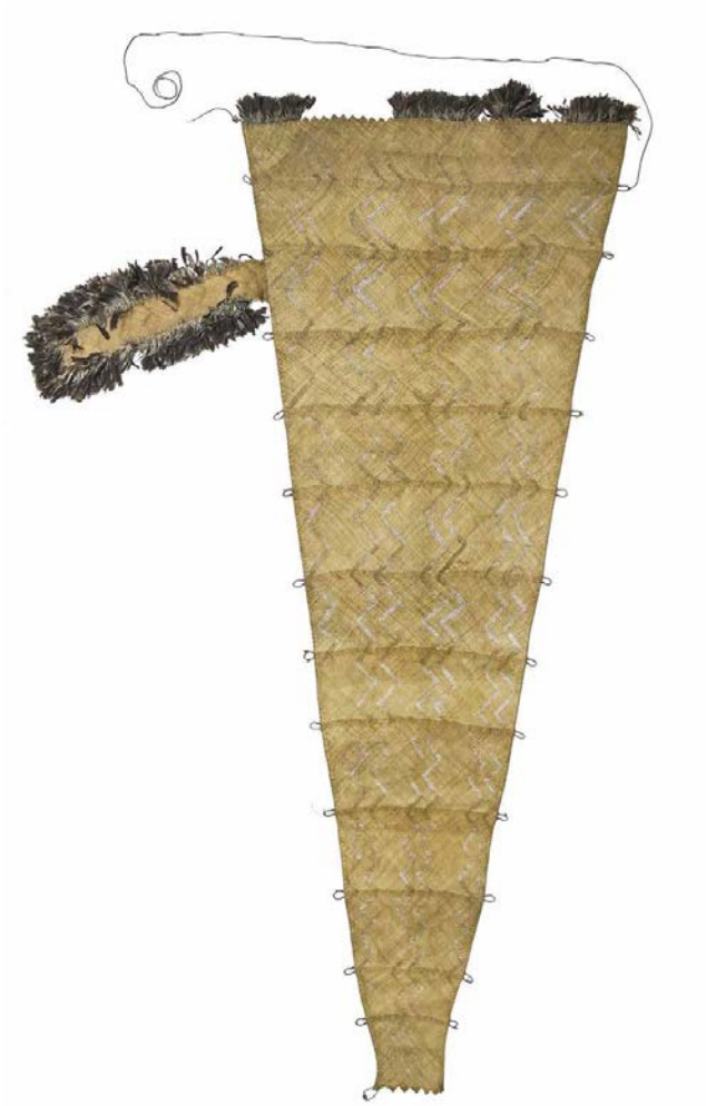
Figure 3. A Māori sail in the British Museum (Oc, NZ. 147), attributed to collection by a Cook expedition. There are loops down both sides of the sail for attachment of two spars, which would intersect below the sail. The leading edge of the sail is to the right and the pennant is attached to the trailing edge on the left, where it served as both a decoration and a “tell-tail”. This sail could have been collected because it is particularly ornate.
