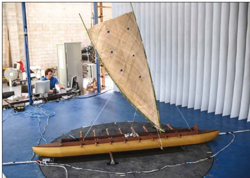
Figure 7. A model canoe in the Twisted Flow Wind Tunnel at the University of Auckland in 2008. In this experiment a 2.8m hull was set up as a single outrigger canoe with a triangular pandanus sail 1.74m high, 0.71m wide at the top, and with a curvature 120mm deep added as an arc to the trailing edge. The model was rotated on a balance which measured forces and moments at 10° intervals and “tell-tails” attached to the sail allowed the trim to be controlled remotely by miniature electric winches. Data were recorded by computer and cameras.
