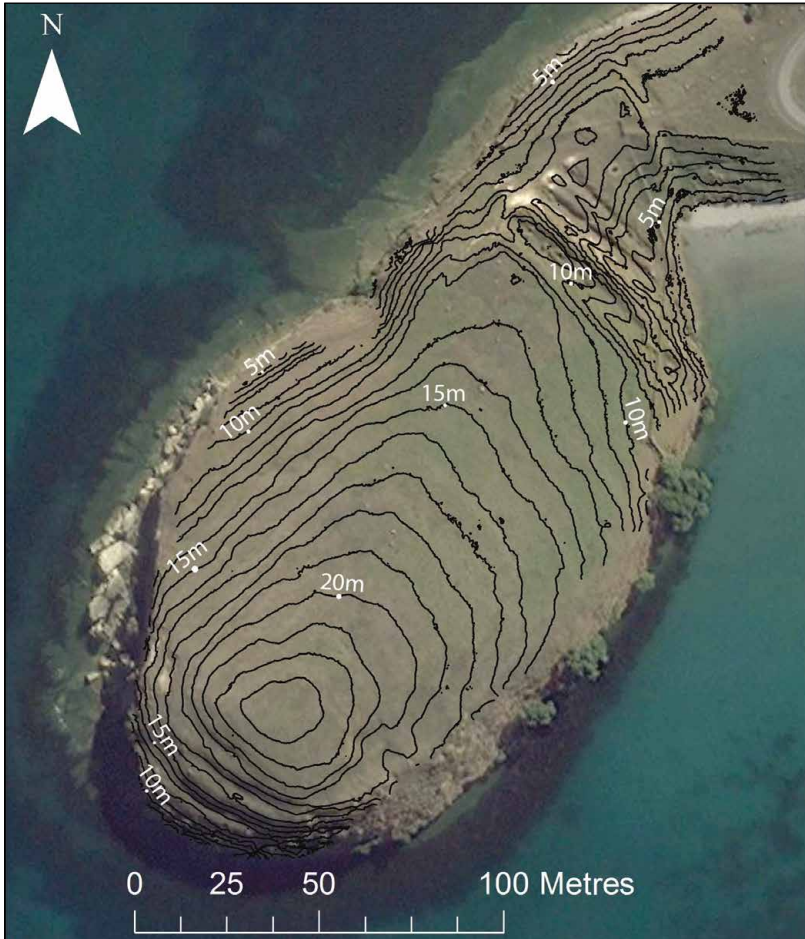
Figure 2. Satellite image of Matakawau Pā with 1 m contours, labelled at 5 m intervals.
