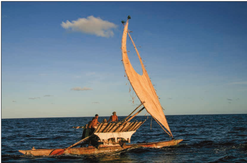
Figure 10. The two “arms” of the sail of a Te Alo Lili in different positions. The leeward head curves to right (leeward) and the windward head curves to left (windward). Photo by M. George.
