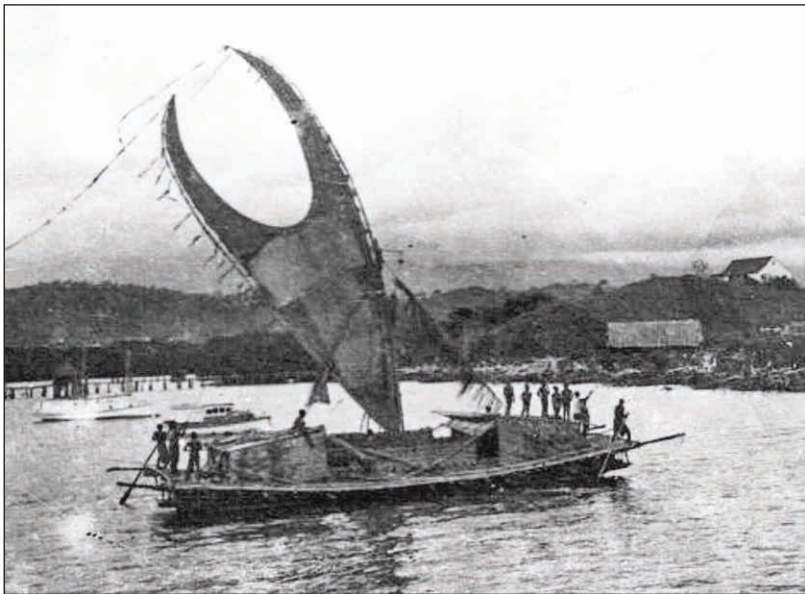
Figure 12. Papua New Guinea lagatoi sails with camber. Note that the body of sail (the undivided part that is under the extended arms of the sail) is longer than the body of a Te Laa o Lata . Photo by an unknown public servant under Hubert Murray, Papua, 1955.
