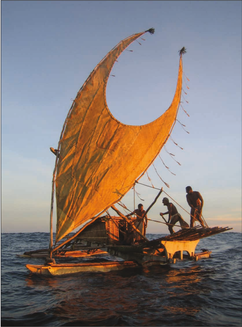
Figure 5. A Te Alo Lili in low wind conditions with its “arms” in a default position. Photo by Wade Fairley.
