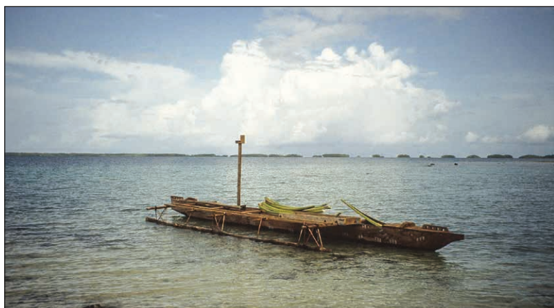
Figure 16. New vaka at anchor. The platform on the stern outrigger booms is for an outboard motor and the raised platform for a lamp to attract flying fish at night. Author's photo, 1991.
