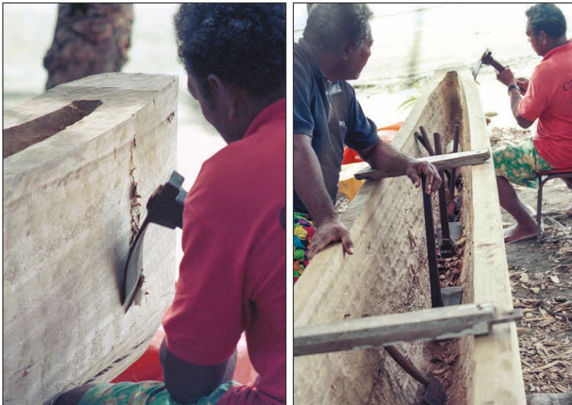
Figure 8 (left and right). Adzing the exterior of the hull. Note the collection of adzes at hand. Photographs by Richard Moyle.
